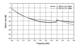
Figure 6. Return Loss vs Frequency. Off Ports
