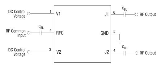
$C_{BL} = 47 \text{ pF for } >1 \text{ GHz operation. Increase}$  value for lower frequency operation.
