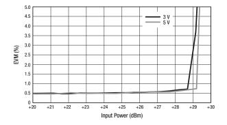
Figure 8. EVM vs Input Power (802.11g 64 QAM, 54 Mbps, f = 2.45 GHz)
