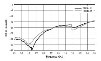
Figure 5. Return Loss vs Frequency, On Ports
