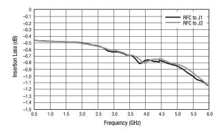
**Figure 3. Insertion Loss vs Frequency**
