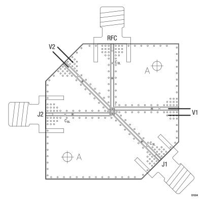
Figure 10. SKY13348-374LF Evaluation Board Assembly Diagram
