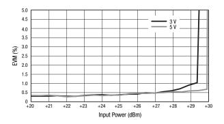
Figure 7. EVM vs Input Power (WiMAX 802.16 64 QAM OFDMA, f = 3.8 GHz)
