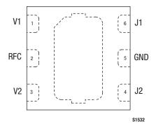
Figure 2. SKY13348-374LF Pinout (Top View)
