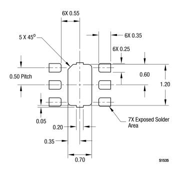
Figure 11. SKY13348-374LF PCB Layout Footprint (Top View)
