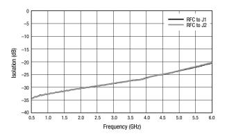
**Figure 4.Isolation vs Frequency**
