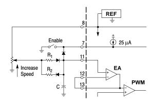
Resistor  $R_1$  with capacitor C sets the acceleration time constant while  $R_2$  controls the deceleration. The values of  $R_1$  and  $R_2$  should be at least ten times greater than the speed set potentiometer to minimize time constant variations with different speed settings.
