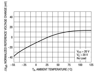
Figure 9. Reference Output Voltage versus Temperature
