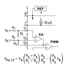
Figure 31. Differential Input Speed Controller
