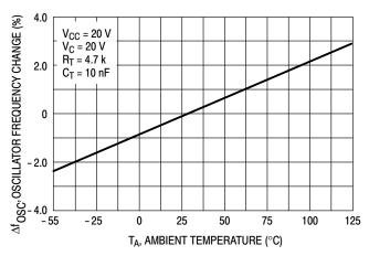
Figure 2. Oscillator Frequency Change versus Temperature
