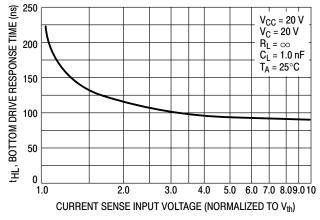
Figure 11. Bottom Drive Response Time versus
