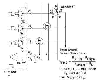
Control Circuitry Ground (Pin 16) and Current Sense Inverting Input (Pin 15) must return on separate paths to the Central Input Source Ground.
