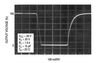
Figure 14. Top Drive Output Waveform
