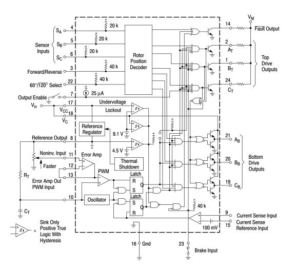
Figure 19. Representative Block Diagram
