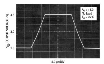
Figure 6. Error Amp Large-Signal Transient Response
