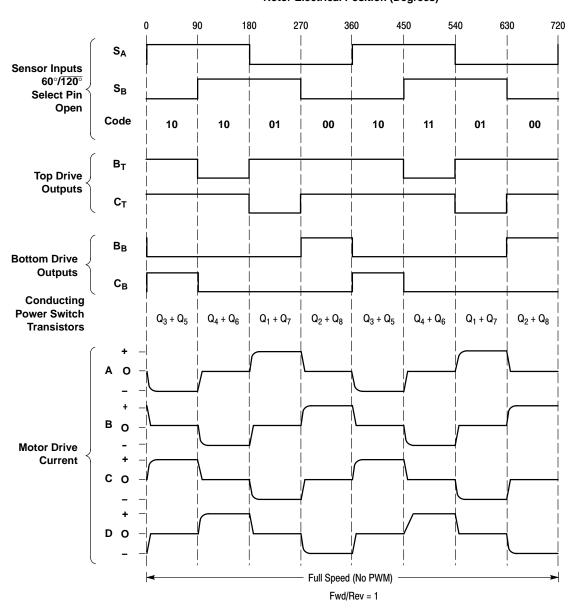
Figure 44. Four Phase, Four Step, Full Wave Motor Controller
