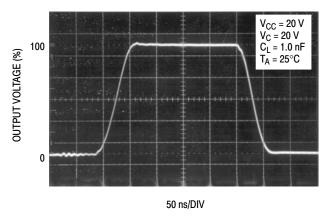
Figure 15. Bottom Drive Output Waveform
