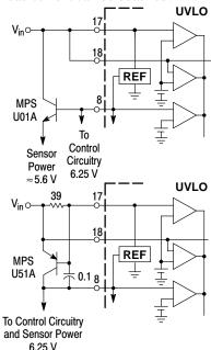
The NPN circuit is recommended for powering Hall or opto sensors, where the output voltage temperature coefficient is not critical. The PNP circuit is slightly more complex, but is also more accurate over temperature. Neither circuit has current limiting
