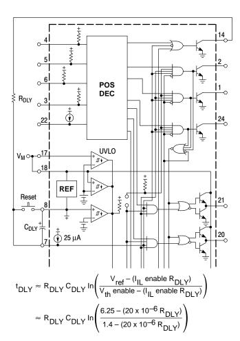
Figure 23. Timed Delayed Latched Over Current Shutdown
