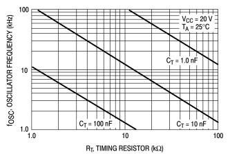
Figure 1. Oscillator Frequency versus Timing Resistor
