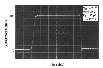
Figure 16. Bottom Drive Output Waveform
