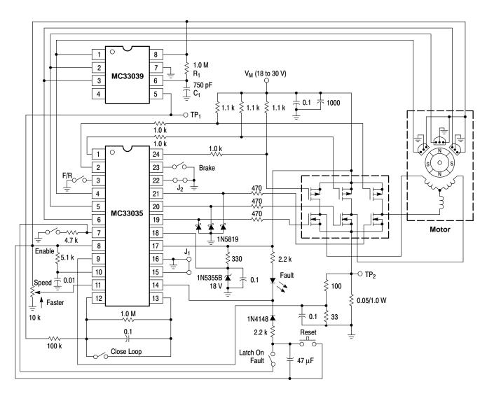
Figure 39. Closed Loop Brushless DC Motor Control Using The MC33035 and MC33039
