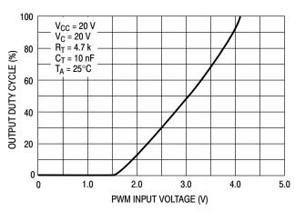
Figure 10. Output Duty Cycle versus PWM Input Voltage
