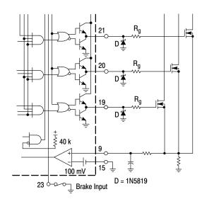
Series gate resistor  $R_g$  will dampen any high frequency oscillations caused by the MOSFET input capacitance and any series wiring induction in the gate–source circuit. Diode D is required if the negative current into the Bottom Drive Outputs exceeds 50 mA.
