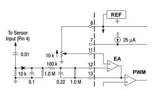
The rotor position sensors can be used as a tachometer. By differentiating the positive–going edges and then integrating them over time, a voltage proportional to speed can be generated. The error amp compares this voltage to that of the speed set to control the PWM.
