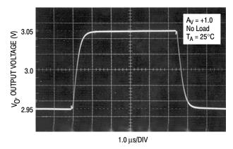
Figure 5. Error Amp Small-Signal Transient Response
