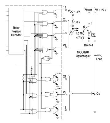
Figure 25. High Voltage Interface with N-Channel Power MOSFETs
