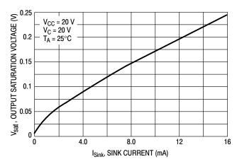
Figure 12. Fault Output Saturation versus Sink Current
