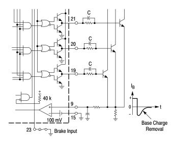
The totem–pole output can furnish negative base current for enhanced transistor turn–off, with the addition of capacitor C.
