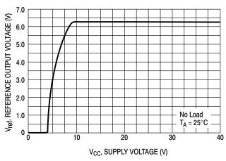
Figure 8. Reference Output Voltage versus Supply Voltage
