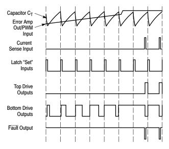
Figure 21. Pulse Width Modulator Timing Diagram Reference
