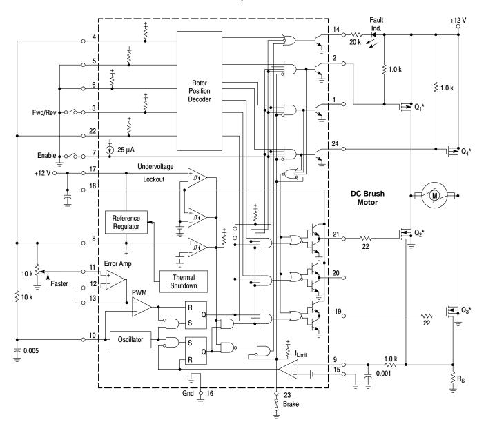
Figure 46. H-Bridge Brush-Type Controller
