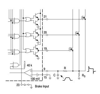
The addition of the RC filter will eliminate current–limit instability caused by the leading edge spike on the current waveform. Resistor  $\mathsf{R}_\mathsf{S}$  should be a low inductance type.
