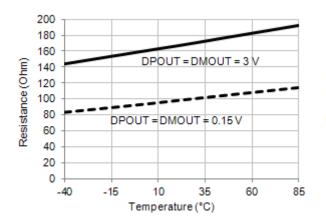
Figure 10.10 Power Switch On Resistance vs. Temp
