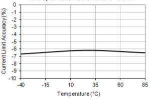
Figure 10.17 IBUS Measurement Accuracy
