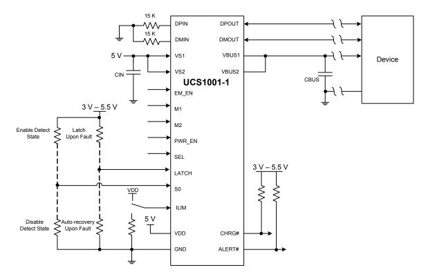
Figure 4.3 UCS1001-1 System Configuration (No USB Host, with Charger Emulation)
