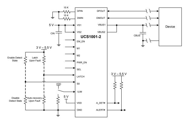
Figure 4.4 UCS1001-2 System Configuration (No USB Host, with Charger Emulation)
