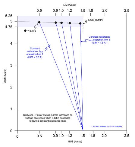
Figure 6.2 Constant Current Limiting (Variable Slope) Operation
