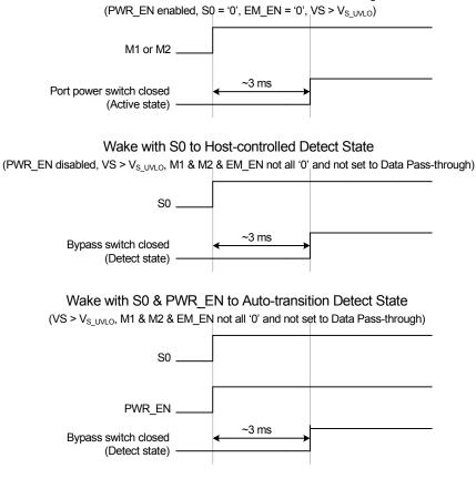
Wake with M1 or M2 to Active State Data Pass-through Mode
