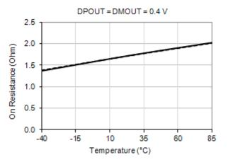
Figure 10.11 R<sub>DCP\_RES</sub> Resistance vs.Temp
