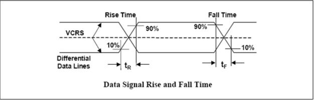
Figure 3.1 USB Rise Time / Fall Time Measurement
