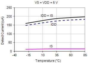
Figure 10.20 Sleep State Current vs. Temp
