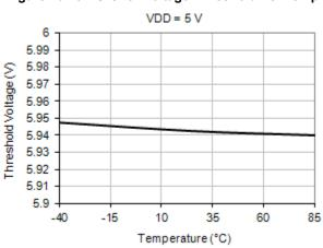
Figure 10.13 VS Over-Voltage Threshold vs. Temp Figure 10.1
