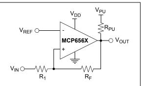
**FIGURE 4-4:** Non-Inverting Circuit with Hysteresis for Single-Supply.
