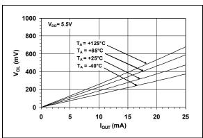
*FIGURE 2-24:* Output Headroom vs. Output Current.
