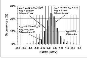
FIGURE 2-41: Common-mode Rejection Ratio (CMRR).
