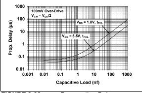
FIGURE 2-32: Propagation Delay vs. Capacitive Load.
