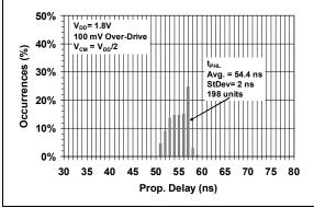
FIGURE 2-25: High-to-Low Propagation Delays.
