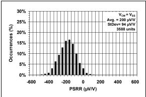
**FIGURE 2-38:** Power Supply Rejection Ratio (PSRR).
