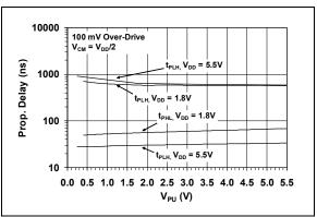
FIGURE 2-36:Propagation Delay vs.Pull-up Voltage.
