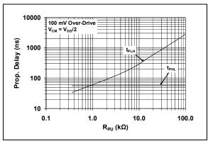
*FIGURE 2-35:* Propagation Delay vs. Pull-up Resistor.
