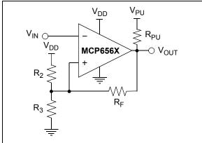
FIGURE 4-6: Inverting Circuit with Hysteresis.
