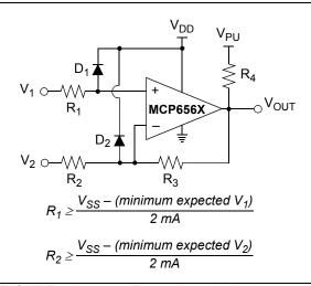
FIGURE 4-3: Protecting the Analog Inputs.
