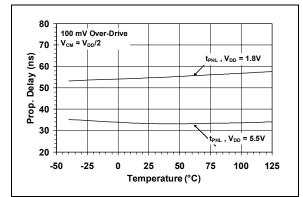
**FIGURE 2-29:** Propagation Delay vs. Temperature.
