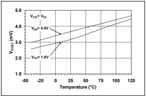
**FIGURE 2-10:** Input Hysteresis Voltage vs. Temperature.
