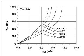
FIGURE 2-21: Output Headroom vs. Output Current.
