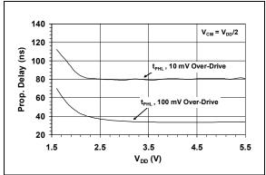
FIGURE 2-27: Propagation Delay vs. Supply Voltage.
