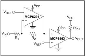
FIGURE 4-12: Precise Inverting Comparator.
