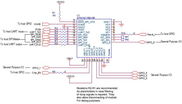
Figure 10-1. SPI Application Schematic
