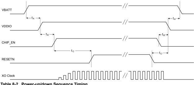
Figure 8-1. Power Up/Down Sequence
